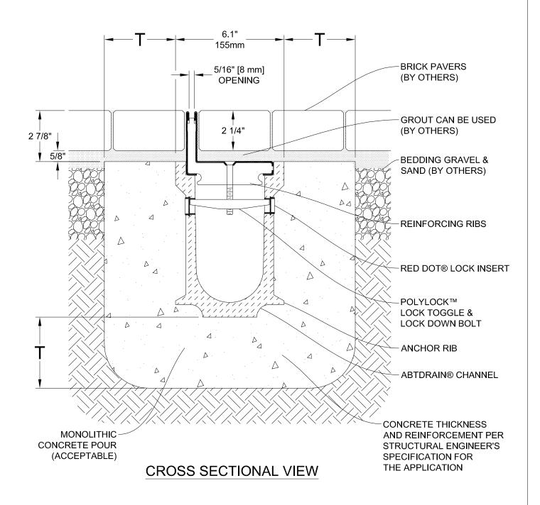
T = FLOOR SLAB THICKNESS, OR 4" [100mm], OR SPECIFICATION (WHICHEVER IS GREATER)
